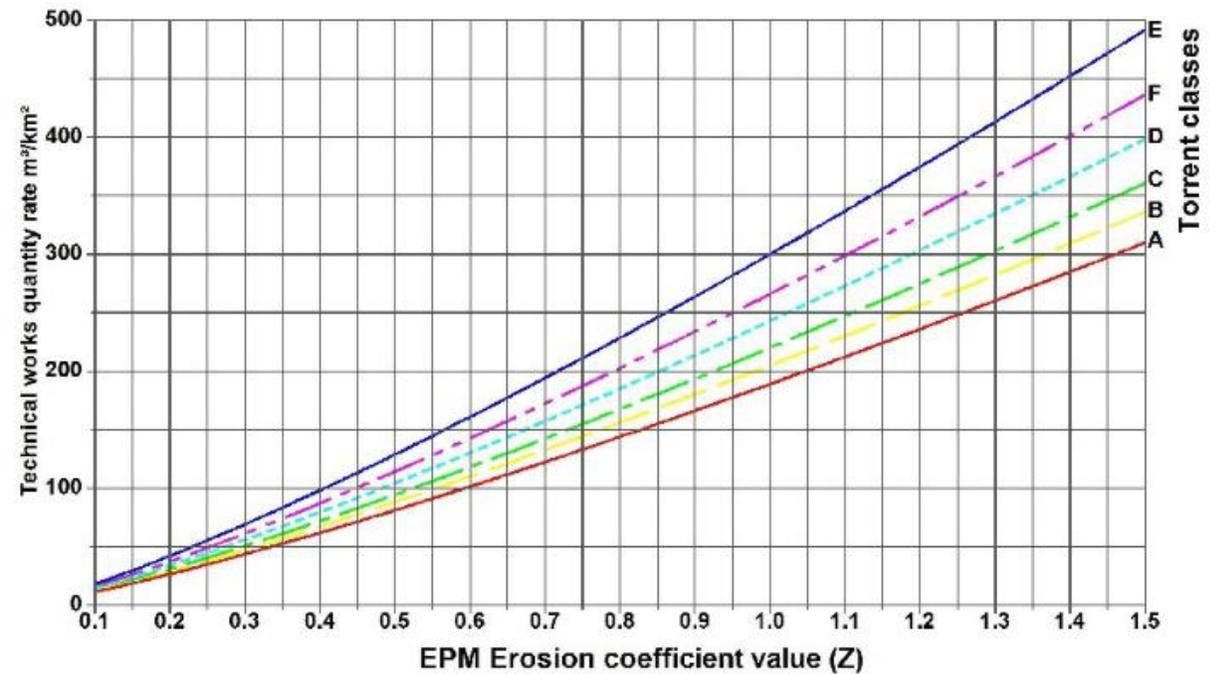
Figure 2. Relations between erosion coefficient and technical works quantity rate
