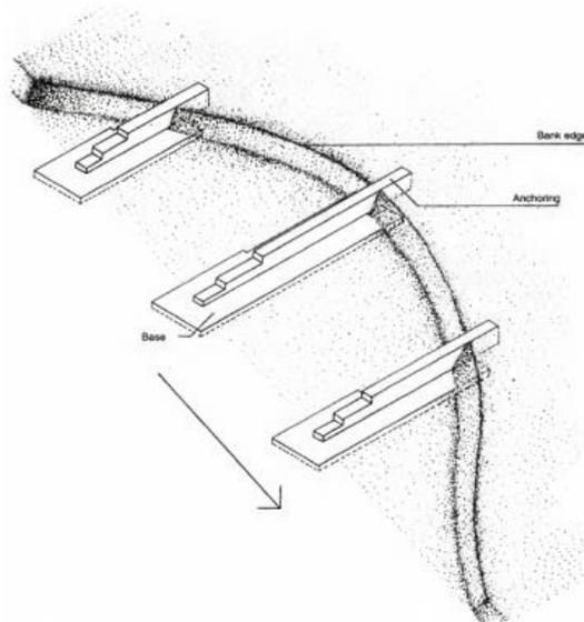
Figure 59. Series of gabion groyne on a gabion base along an eroded bank
