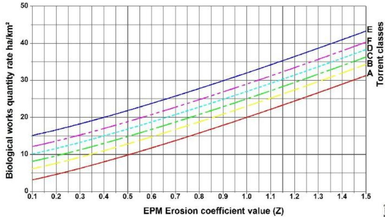
Figure 1. Relations between erosion coefficient and biological works quantity rate
